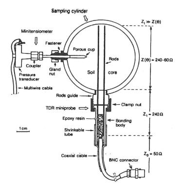
Fig. 1. Cross-section of the 'measuring cell' with the TDR soil moisture miniprobe installed. Also the minitensiometer is shown in details. Discontinuities of the miniprobe impedance are marked with dashed line.
