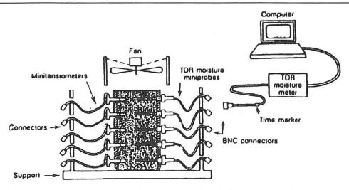
Fig. 2. Structural setup of the experimental stand. A soil core under investigation is kept in a metal sampling cylinder. An array of five minitensiometers and another array of five TDR soil moisture miniprobes are installed, marking of five independently monitored layers of the soil. Spiral arrangement of the probes is not visualized.
